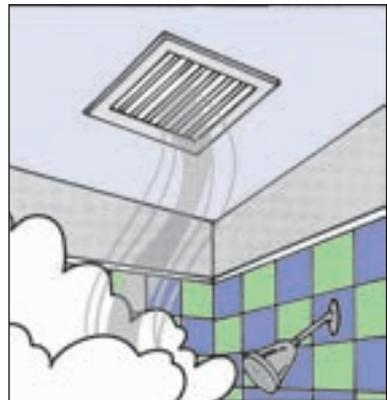
**\*Caution:** when using large exhaust fans, combustion appliances with chimney may not operate properly.
